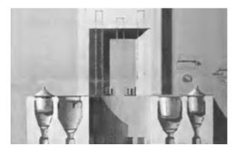
Fig 4. Vertical section of a kitchen fire-place in the house of Baron Lerchenfeld in Munich designed by Count Rumford, ca. 1870
